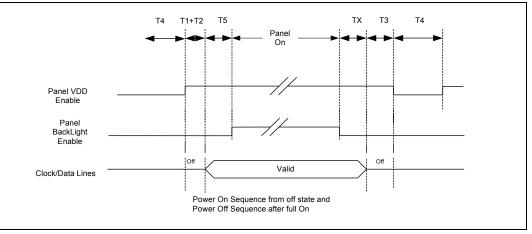
**NOTE:** Support for programming parameters TX and T1 through T5 using software is provided.
