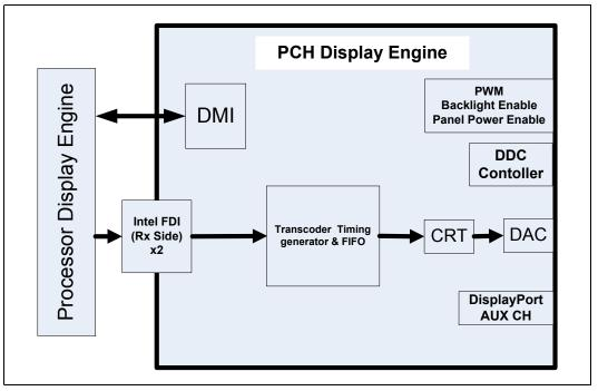
The PCH Analog Port uses an integrated 180 MHz RAMDAC that can directly drive a standard progressive scan analog monitor up to a resolution of 1920x2000 pixels with 24-bit color at 60 Hz with reduced blanking.
