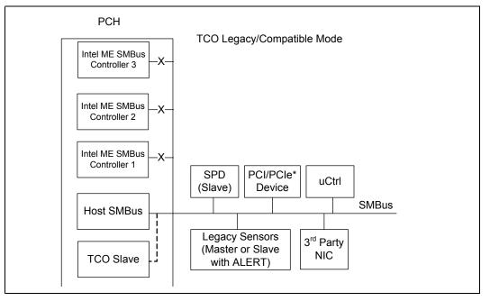
In TCO Legacy/Compatible mode the PCH can function directly with an external LAN controller or equivalent external LAN controller to report messages to a network management console without the aid of the system processor. This is crucial in cases where the processor is malfunctioning or cannot function due to being in a low-power state. Table 5-40 includes a list of events that will report messages to the network management console.
